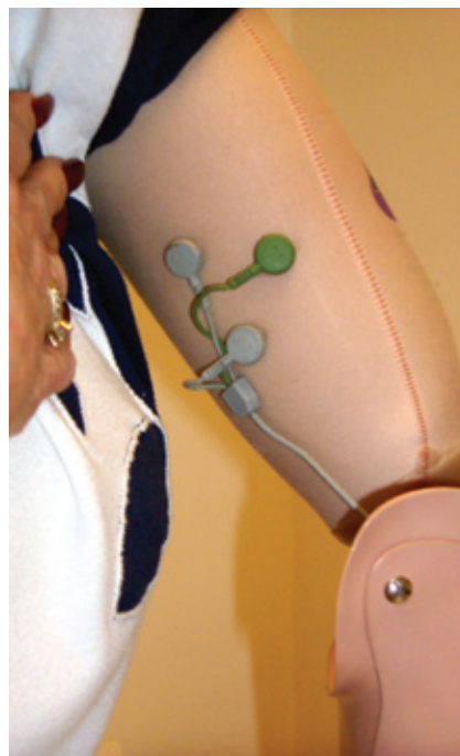
Illustration 4 Shielded cables and electrodes.
